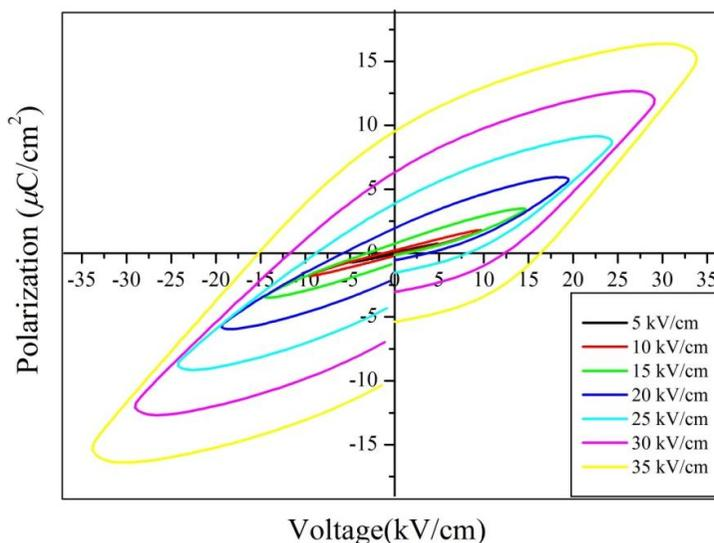
**Figure 5** P-E hysteresis loop of BNT-BKT-BT ceramic sintered at 1175 °C.
