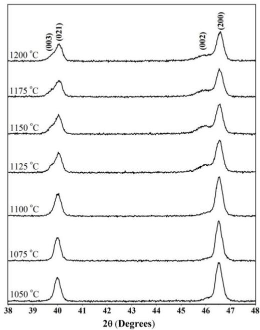
**Figure 2** X-ray patterns of BNT-BKT-BT ceramic in the  $2\theta$  range of  $38^\circ$  to  $48^\circ$ .
