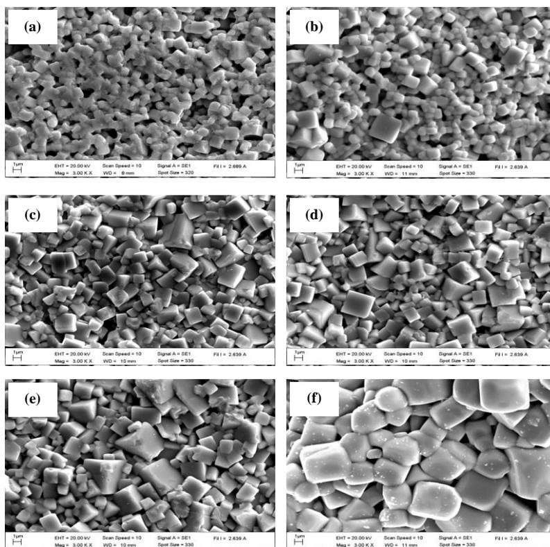
**Figure 3** SEM photographs of BNT-BKT-BT ceramics sintered at; (a)  $1075$  °C, (b)  $1100$  °C, (c)  $1125$  °C, (d)  $1150$  °C, (e)  $1175$  °C and (f)  $1200$  °C.
