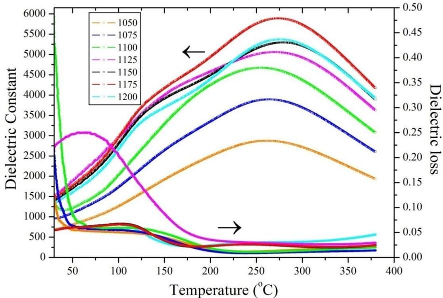
**Figure 4** Temperature dependence of the dielectric constant and dielectric loss tangent of BNT-BKT-BT ceramics measured at 10 kHz.
