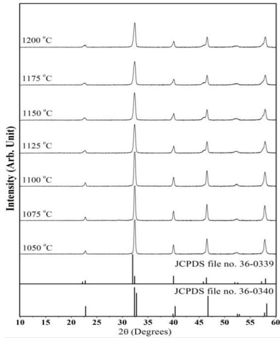
**Figure 1** X-ray patterns of BNT-BKT-BT ceramic at various sintering temperatures in the  $2\theta$  range of  $10^\circ$  to  $60^\circ$ .
