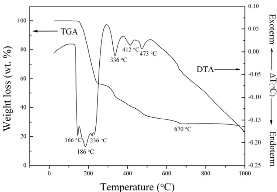
**Figure 2** DTA-TG curves of uncalcined PT powders.
