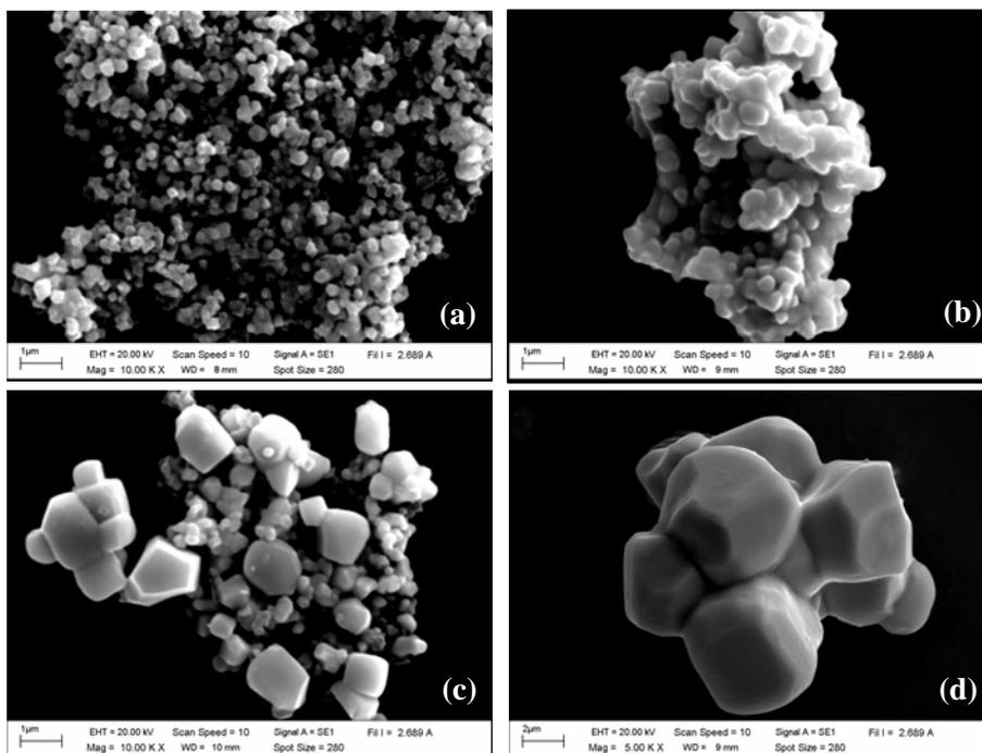
**Figure 6** SEM morphology of PT powders calcined at (a) 600 °C, (b) 700 °C, (c) 800 °C and (d) 900 °C.
