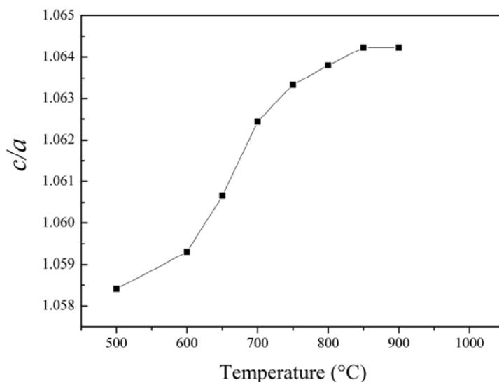
**Figure 5** The  $c/a$  ratio of PT powders with various calcination temperatures.
