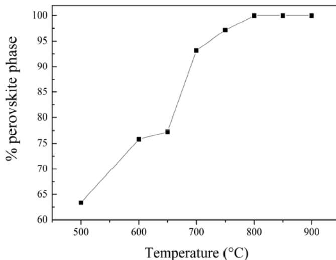
**Figure 4** The percent perovskite phase of PT powders with various calcination temperatures.
