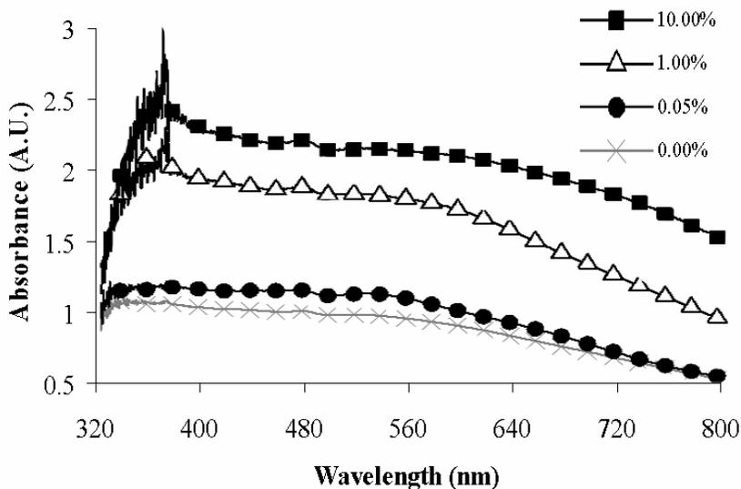
**Figure 2** Optical absorption spectra of ZnO-MWCNTs electrode at different MWCNTs loadings.
