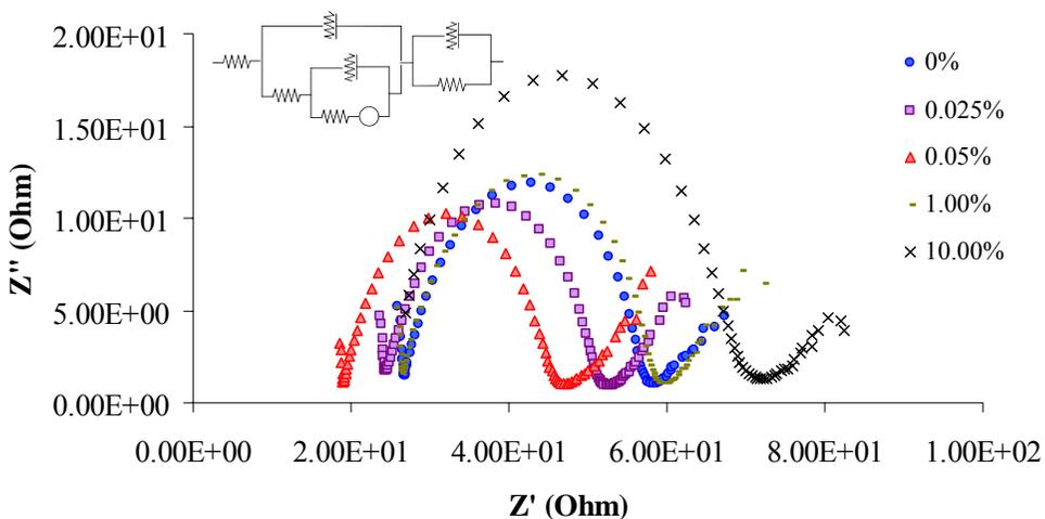
**Figure 3** Nyquist plots of DSSCs with ZnO-MWCNTs electrode at different MWCNTs loadings. In set: the equivalent circuit model of DSSCs based ZnO-MWCNTs electrodes.
