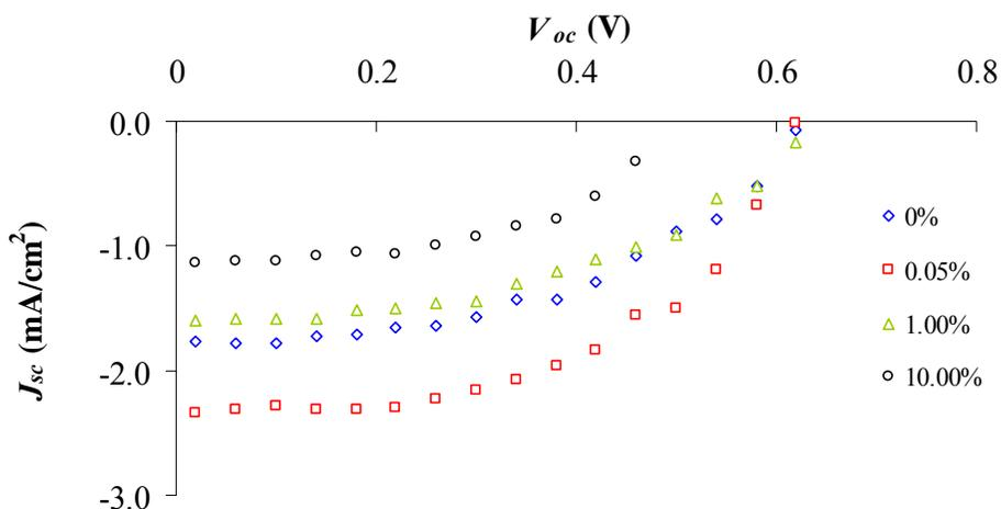
**Figure 4**  $J$ - $V$  characteristics of the ZnO-MWCNTs front electrode of the DSSCs
