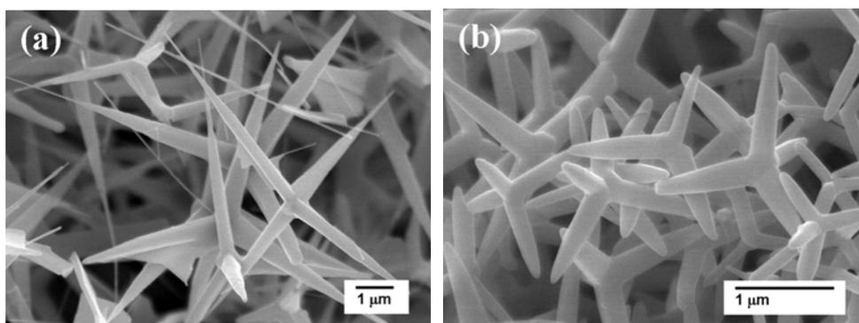
**Figure 1** FE-SEM images showed two different shapes of the tetrapods, (a) sharp tip and (b) round tip.
