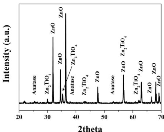
**Figure 3** XRD pattern of the tetrapods scanning for  $2\theta$  in rang of 20-70°, showing ZnO phase with small amount of  $Zn_2TiO_4$  and anatase- $TiO_2$  phases.
