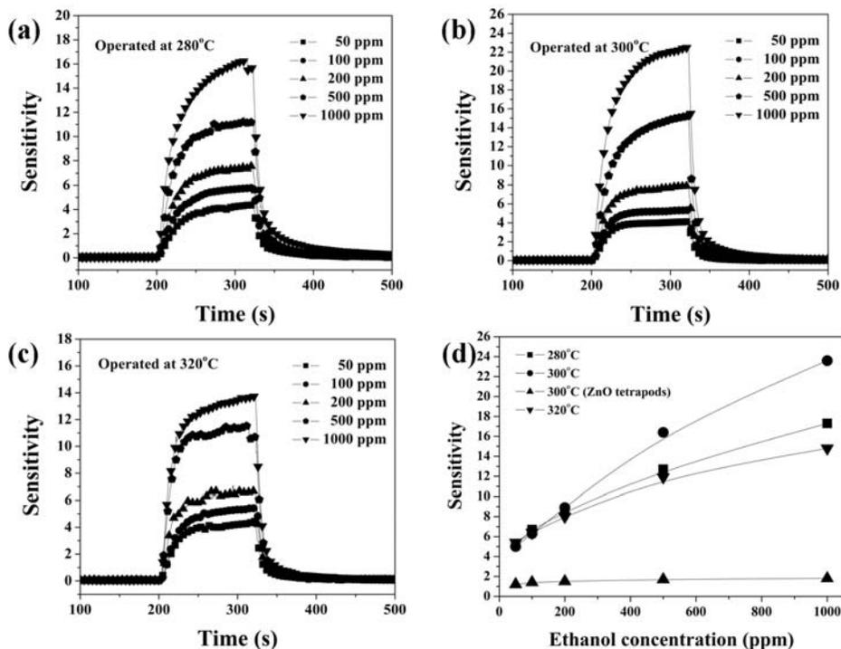
**Figure 4** Sensitivities of sensor operated at (a) 280°C, (b) 300°C, (c) 320°C, and (d) the sensor sensitivity in (a-c) compared with pure ZnO tetrapods sensor.
