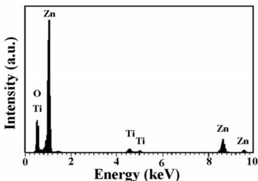
**Figure 2** EDS spectrum performed on one leg of tetrapod indicated that the tetrapod consisted of Ti, O, and Zn elements.
