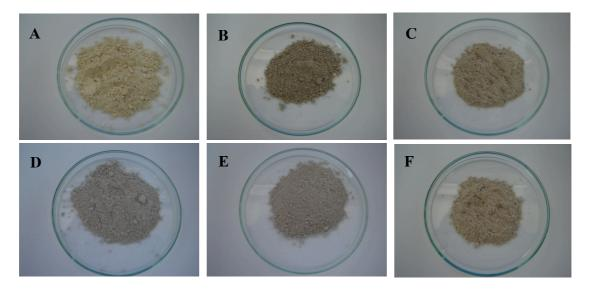
Fig.2 Effect of NaOH concentration on recondition of spent kaolin (A), 0.5 M (B), 1.0 M (C), 1.5 M (D), 2.0 M (E) and 2.5 M (F).
