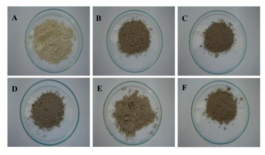
Fig.1 Effect of temperature on characteristic of pure kaolin (A), spent kaolin (B), kaolin reconditioned at  $50^{\circ}$ C (C), kaolin reconditioned at  $70^{\circ}$ C (D), kaolin reconditioned at  $90^{\circ}$ C (E), and kaolin reconditioned at  $100^{\circ}$ C (F).
