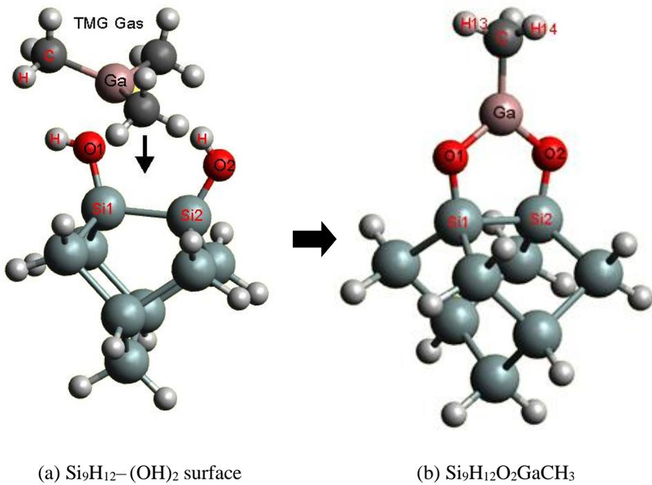
**Figure 4** The possibility of TMG adsorption on the silicon surface as  $\text{Si}_9\text{H}_{12}\text{O}_2\text{GaCH}_3$ .
