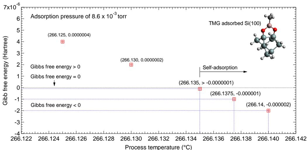
**Figure 5** The possible chart of the relationship between process temperature and Gibbs free energy.
