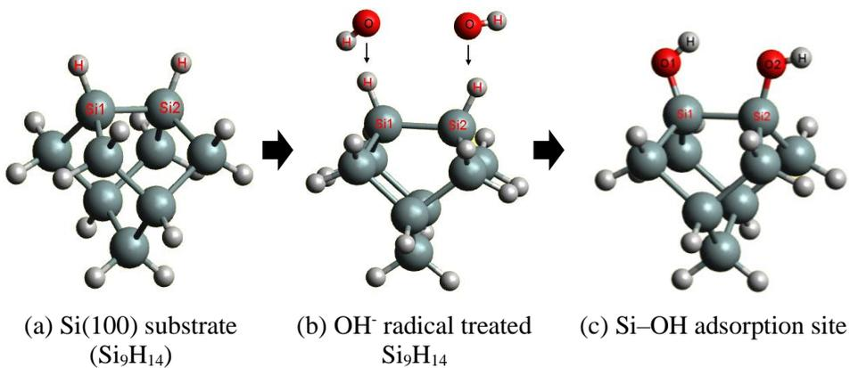
**Figure 3** Production process of surface adsorption site in ALD.
