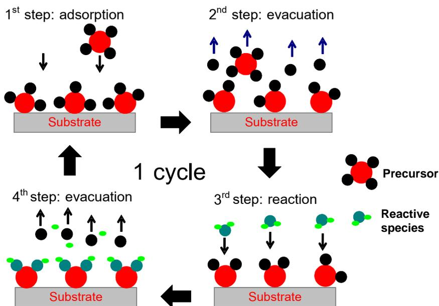
**Figure 1** Basic model for 1 cycle in ALD process
