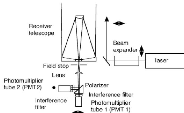
**Figure 1** Block diagram of NIES Mie scattering LIDAR (Sugimoto, 2001).
