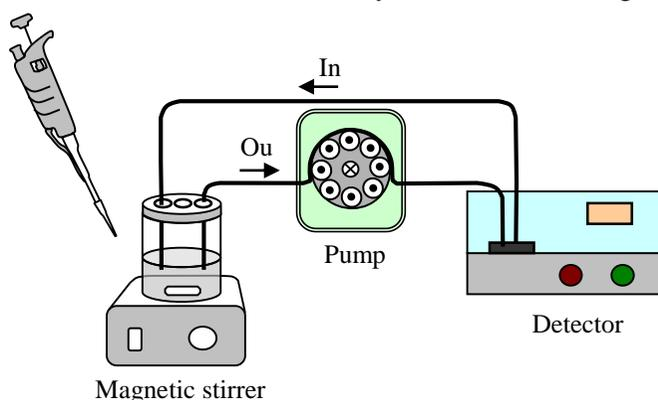
Figure 1. The apparatus for small scale mole ratio determination and photometric titration
